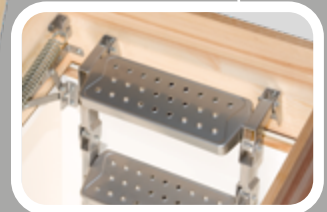
In order to facilitate accessing the attic, the attic ladder's box has been equipped with an additional step which reduces the distance between the last tread of the ladder and the attic floor.
